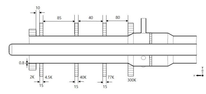
Figure 7. Scheme of a prototype power coupler for thermal analyses
