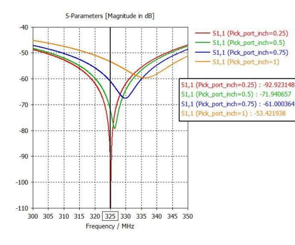
Figure 5. Effect of pick-up port diameter change
