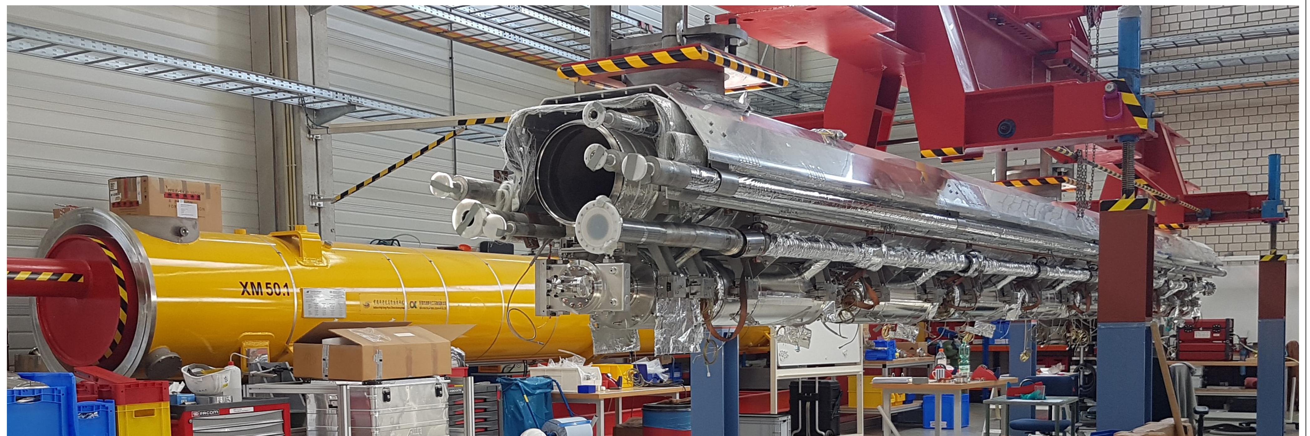
Reassembly of accelerating module XM50.1 (former XM50) in the Accelerator Module Test Facility AMTF
