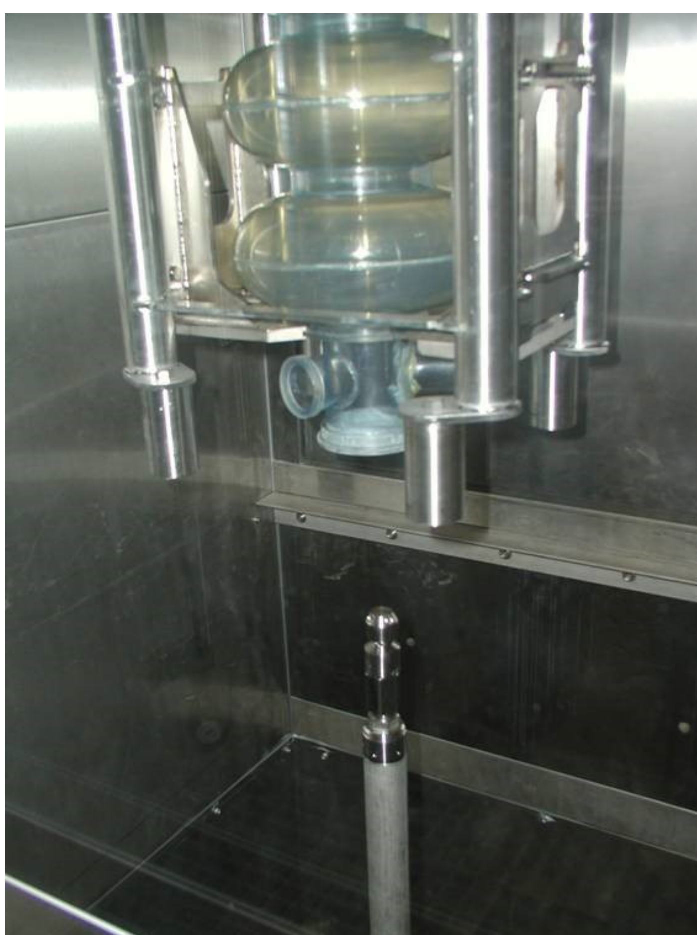
High pressure ultra-pure water rinsing (HPR) setup with acrylic plastic cavity model installed above the sprayhead
