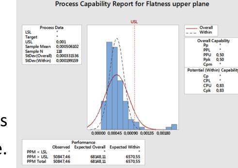
Flatness of reference A has a **Cpk = 0.83**. It is greatly affected by the parts out of tolerance.
