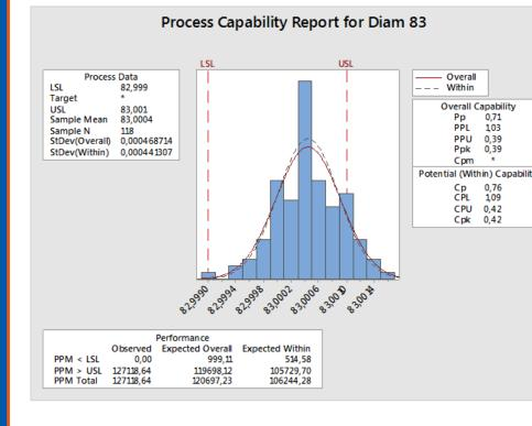
Ø83 mm has a **Cpk = 0.42** which can be translated into 106244 PPM.
