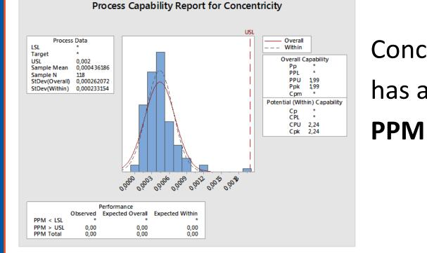
Concentricity of the iris and external diameter has a Cpk shows an impressive **2.24** hence **0**
