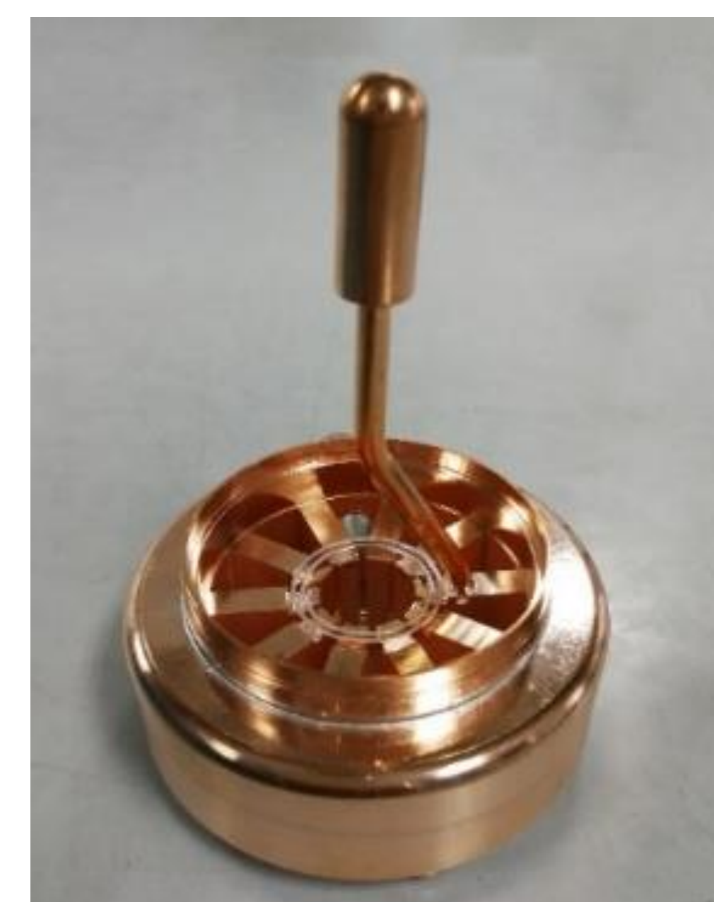
The finished cavity and output antenna
