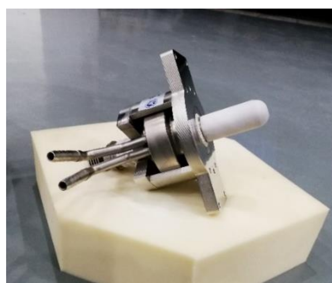
The prototype of 1.5GHz CW magnetron
