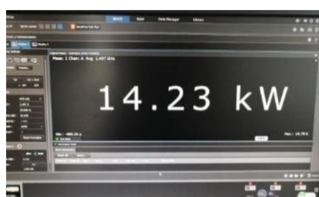
Testing results of 1.5GHz CW magnetron
