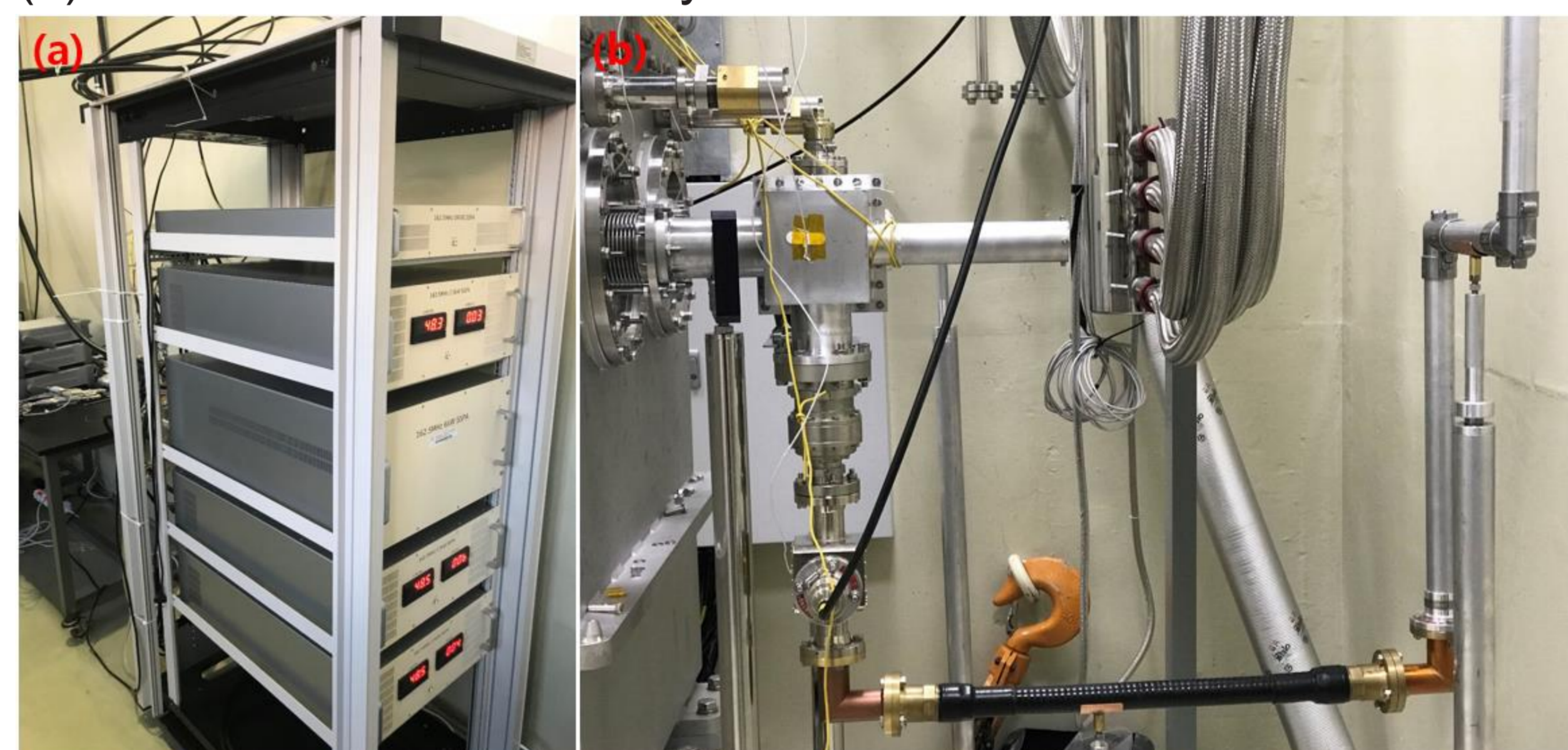
Figure 5: RF test of a HWR cryomodule for (a) SSPA and (b) connection of a coaxial line to an input coupler in the cryomodule. The solid state power amplifier (SSPA) has the drive frequency of 162.5 MHz, continuous-wave (CW) operating mode and the maximum power of 7 kW.
