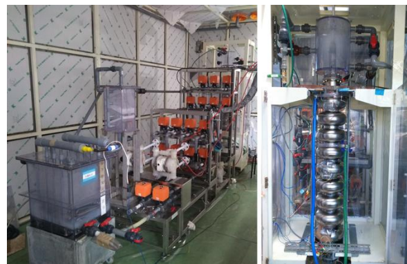
Figure 1: VEP system with auto-valves (left) and cavity set at VEP stand (right) for the VEP process.
