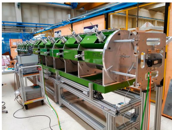
Figure 3: Aluminum DTL with bead pull system, movable tuners and post couplers (courtesy of CERN-Linac4) and VNA.
