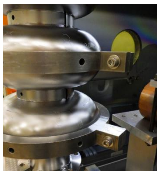
Figure 4: Special jigs set at equator for EBW.
