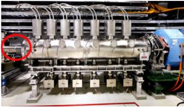
Figure 6: One of 2 extraction kicker magnet sets, with space indicated (red) for an extra magnet placement.
