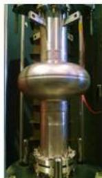
**Nb<sub>3</sub>Sn offers the potential for a high gradient machine operating at 4.2 K**
