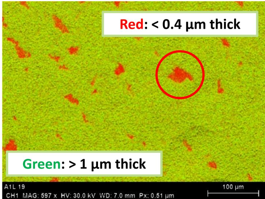
⇒ Solution: Pre-anodising substrate before coating suppresses formation of these thin-film regions!
