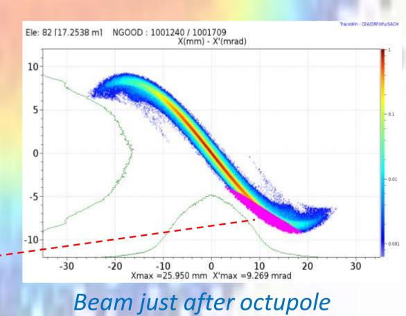
The required octupole to get a flat beam is much weaker in the lower phase advance (1600 T/m<sup>3</sup>) than in the close to  $n\pi$  configuration (2400 T/m<sup>3</sup>).
