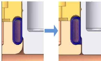
Previous (on left) and new (on right) cathode spring design: the new design has been optimized to avoid any sharp edges [1].
