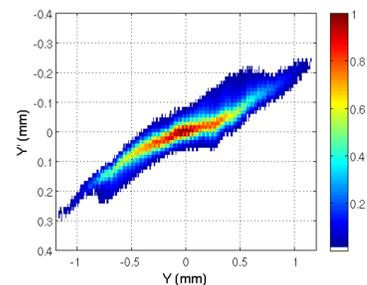
Horizontal (on top) and vertical phase space measured for a 0.5 nC electron beam after optimization. Despite the rotational symmetric injector, horizontal and vertical phase space are different. To explain this, investigation are on going (see poster MOPLR013).
