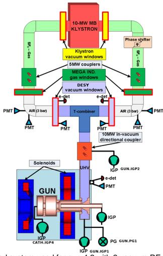
RF feed system used for gun 4.2 with 2 vacuum RF windows. Main interlock (IL) systems:
