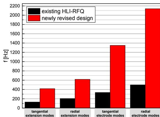
Figure 7: Mechanical electrode resonance frequencies of the existing HLI-RFQ and the newly revised design
