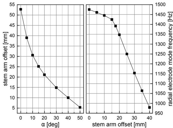
Figure 2: Required stem arm offset for full dipole compensation as function of the stem cutting angle  $\alpha$  (left) and mechanical radial electrode mode frequency as function of the stem arm offset (right).
