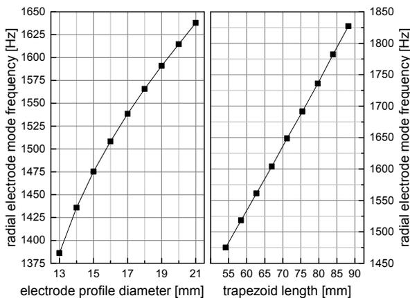
Figure 3: Radial electrode mode frequency as function of the electrode profile diameter (left) and base length of the trapezoidal mounting (right).
