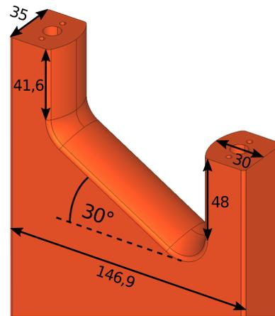
Figure 5: Reinforced stem geometry.
