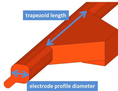
Figure 4: Electrode profile diameter and length of the trapezoidal electrode mountings.
