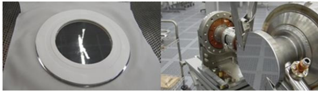
Figure 5: Beam pipe cover for LCLS-II prototype cavity string assembly.
