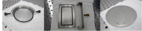
Figure 1: Stainless steel covers with O-ring (left, middle) and niobium blank (right).
