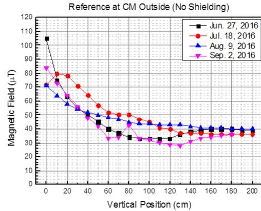
Figure 5: Geomagnetic field distribution measured at the QWR cryomodule outside.
