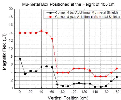
Figure 8: Comparison of geomagnetic field distribution with and without the additional Mu-metal shields.
