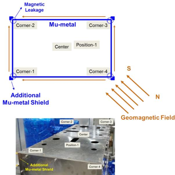
Figure 7: Schematic of the magnetic leakage and a photograph on the measurement positions.
