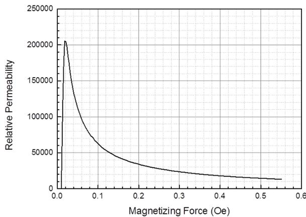
Figure 3: Relative permeability measured for a Mu-metal sample reannealed with hydrogen supply.
