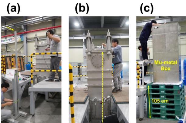
Figure 4: Geomagnetic field measurements at (a) the QWR cryomodule outside, (b) the cryomodule inside, and (c) the Mu-metal box inside.
