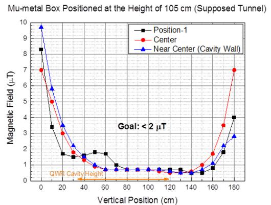
Figure 6: Geomagnetic field distribution measured in the Mu-metal box.
