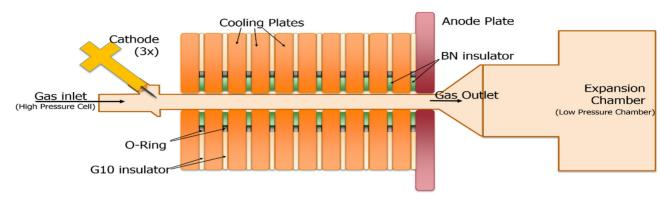
Figure 1: Schematic (not to scale) of the Plasma Window. Ten cascaded arc cooling plates of floating potential are each 1 cm in width and separated by 1mm of O-ring, boron-nitride spacers, and G10 spacers to insulate them from their neighbors. Three thoriated tungsten needle cathodes collectively deliver up to 90 amps.
