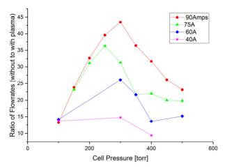
Figure 3: Ratio of flowrates (arc OFF to arc ON) as the cell (inlet) pressure is varied between 100 and 500 torr, for multiple current values. 90 A and 75 A curves show a shifting of the maximum ratio. There is a current lack of data points for 60 A and 40 A in expected pressure range to indicate continuation of shift.
