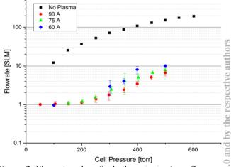
Figure 2: Flowrate values for both un-ionized gas flow an plasma at multiple current values. Error bars are the stand ard deviation of all points (between 50 and 150 points) during the collection time for a specific pressure setpoint.
