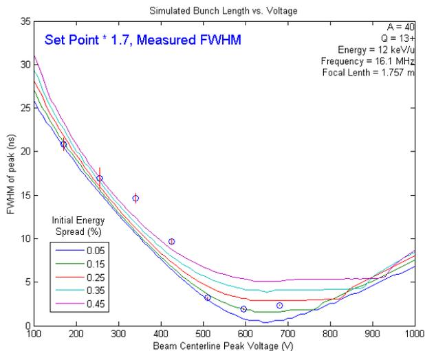
Figure 2: Measured pulse widths overlaid on simulated FWHM vs. voltage curves for the 16.1 MHz mode.
