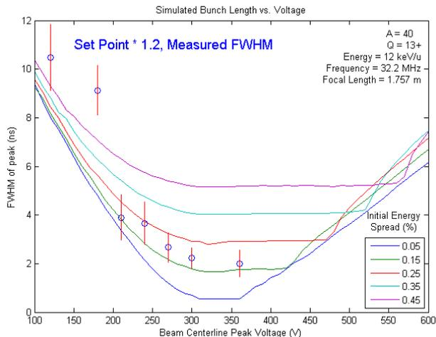
Figure 3: Measured pulse widths overlaid on simulated FWHM vs. voltage curves for the 32.2 MHz mode.
