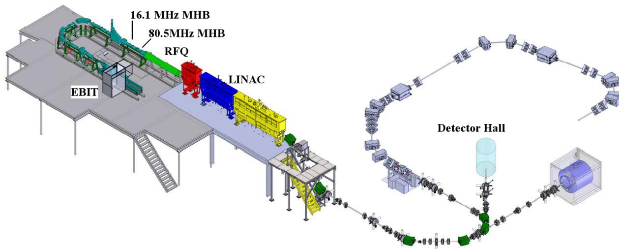
Figure 1: Layout of the NSCL ReAccelerator, including the location of the 16.1 MHz buncher.
