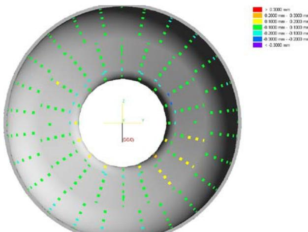
Figure 4: Results of 3D-measurements of cavity half-cell.
