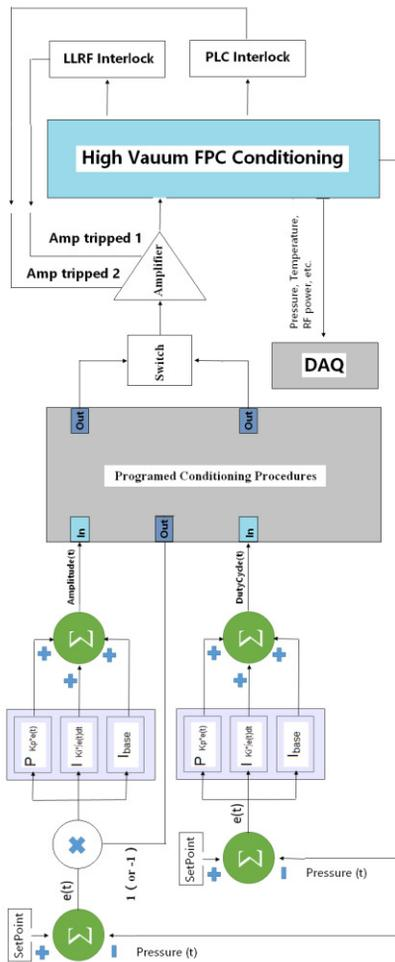
Figure 2: Diagram of new conditioning system.
