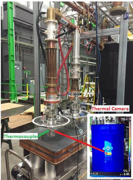
Figure 4: First section of comparison test with original design FPCs.
