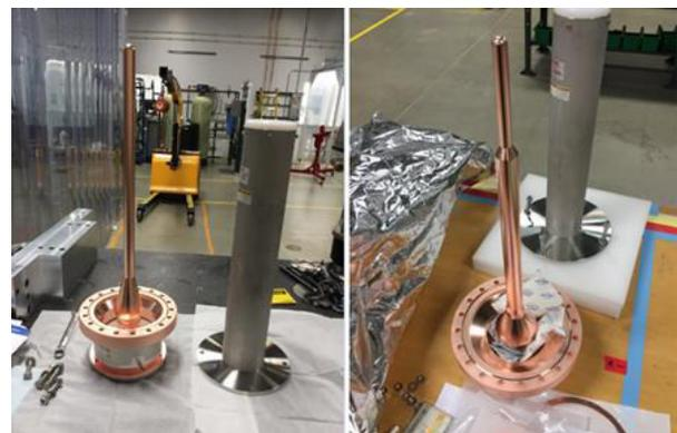
Figure 3: Pictures of IC prototypes (left one is original design, right one is multipacting-free design).
