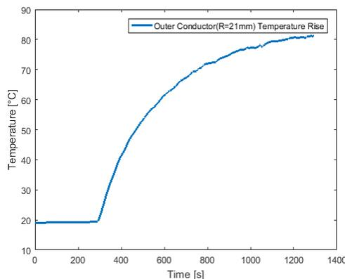
Figure 5: Temperature rise of original coupler's outer conductor (R=21mm).
