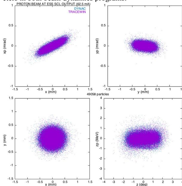
Figure 4: Phase space portraits for TRACEWIN and DYNAC at the ESS SCL output.
