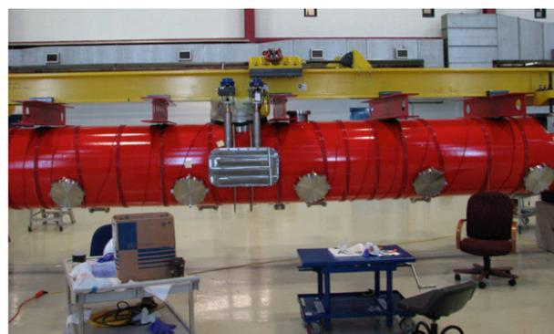
Figure 4: This is a picture of the cryomodules at FNAL that is ready to be demagnetized. The solenoid coil is wound around the CM for the demagnetization process.
