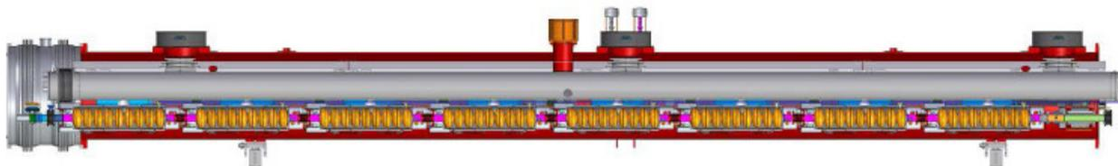
Figure 2: The LCLS-II 1.3 GHz Cryomodule.
