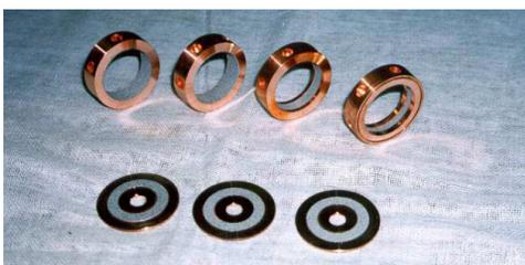
Figure 4: The components of the load with absorbing material.
