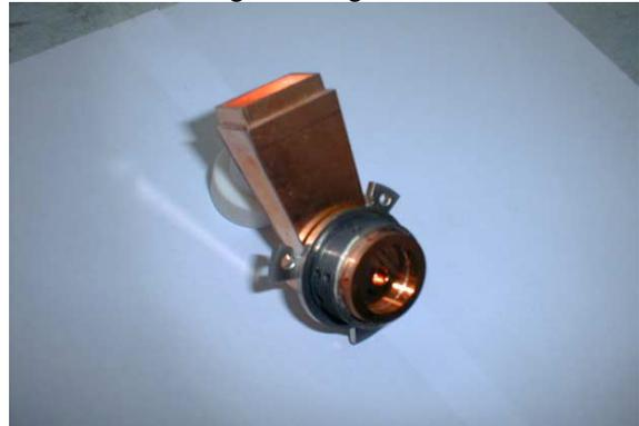
Figure 1: RF input coupler assembly.
