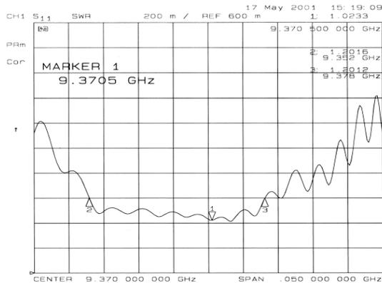
Figure 7: The measurement results of VSWR vs frequency.
