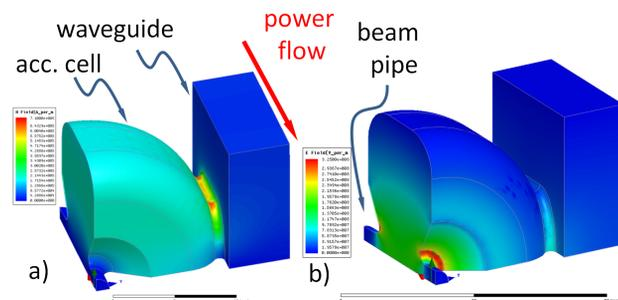
Figure 3: Quarter-cell finite element model of the proposed traveling wave accelerating structure. Surface electric fields are normalized to 100 MV/m accelerating gradient: a) magnetic fields with peak magnitude of 0.71 MA/m; b) electric fields with peak magnitude  $\sim 325$  MV/m.
