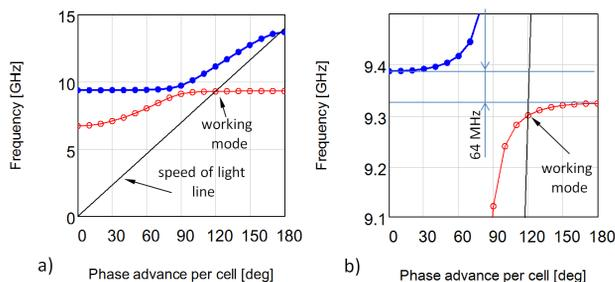
Figure 4: Dispersion diagram for one cell of the TW structure shown in Fig. 4: a) full frequency span with two lowest branches; b) 400 MHz frequency span.
