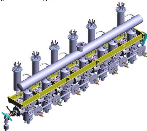
Figure 8: 3D view of the cavity and solenoid string in low beta cryomodule.
