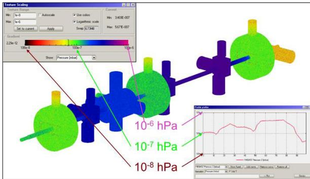
Figure 4: Nitrogen gas pressure diagram in the MEBT.
