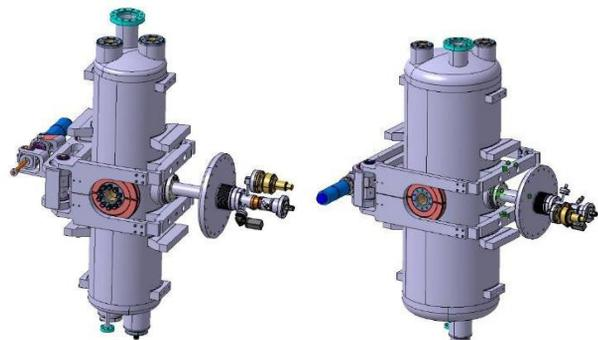
Figure 6: low-beta (left) and high-beta (right) fully equipped cavities.
