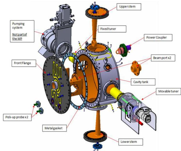
Figure 5: Rebuncher split spoke geometry.
