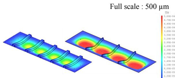
Figure 9: Top plate simulations with Cast3M.
