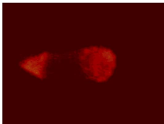
Figure 8: TV camera downstream of kicker which captured a triangularly shaped beam shaped by the sextupole moment inherent in the fields due to the stripline voltages.
