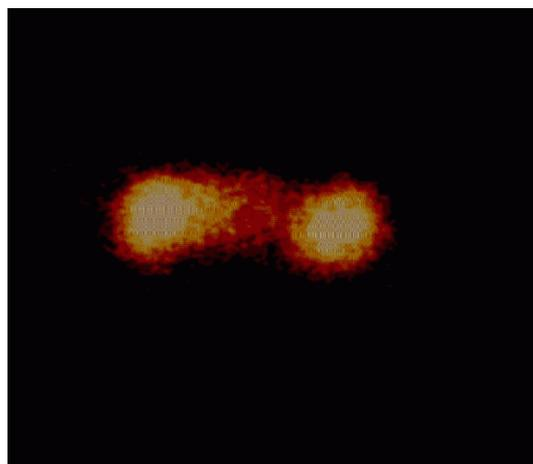
Figure 7: TV camera downstream of kicker which captured the beam as it deflected from one side to the other.
