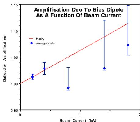
Figure 6:  $x$  displacement at BBT09 (old beam line) due to dipole magnet
