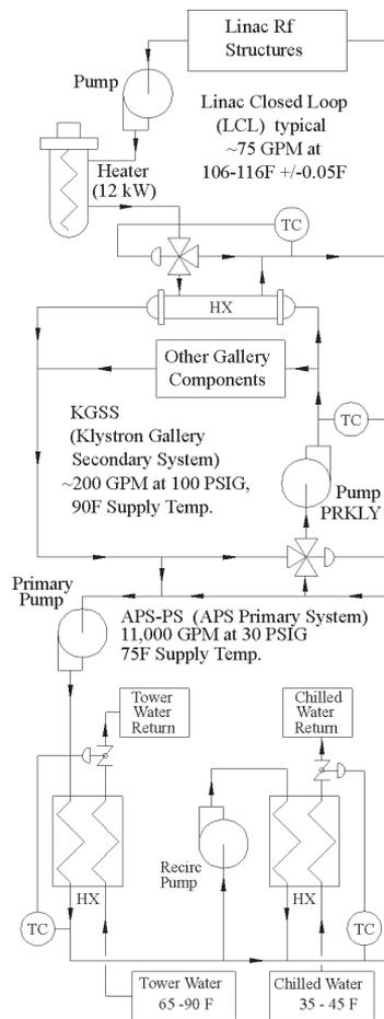
Figure 2: Overview of the linac water system.
