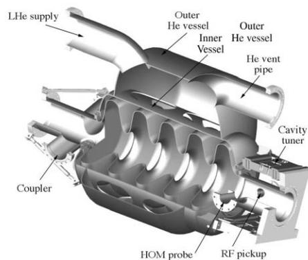
Figure 1: Illustration of  $\beta = 0.64$  cavity design.
