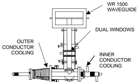
Figure 4: Coaxial Power Coupler
