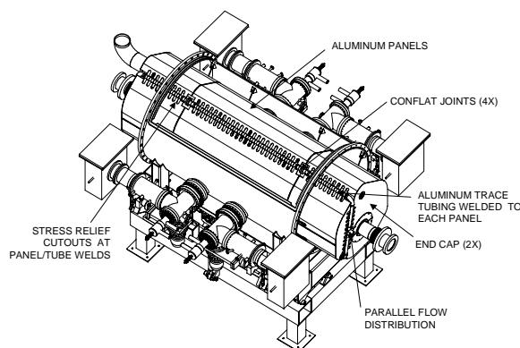
Figure 2: Complete RF Section with heat shield installed.
