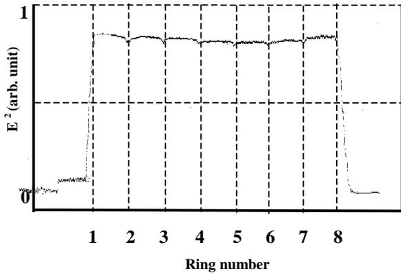
Figure 3: Measured field distribution along 8 ring assembly
