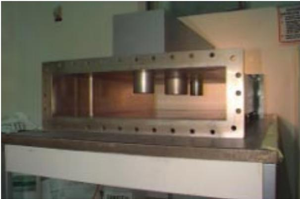
Figure 2: Photograph of 350 MHz WR2300 half-height Phase Shifter.
