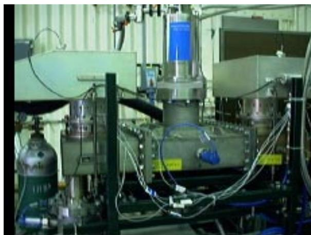
Figure 2: RF Window Pair on the Test Stand
