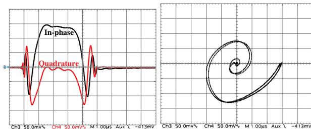
Figure 5: I-Q demodulation results without the phase compensation. Figure 6: I-Q display without the phase compensation.
