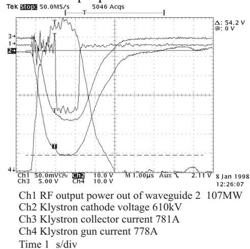
Figure 2: Waveforms at a voltage of 610kV
