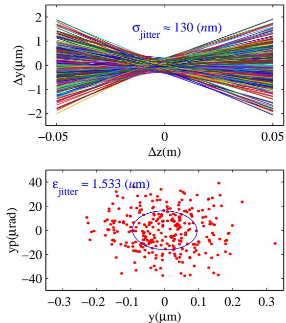
Figure 2. The top plot displays the measured beam trajectories. The bottom plot shows the calculated jitter emittance.
