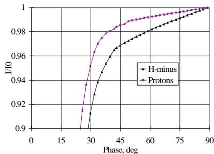
Figure 3: Particle fraction as a function of phase half-width for  $H^-$  and proton beams.
