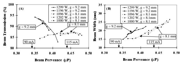
Figure 4. (A) Shows the increased beam transmission from DC1 (ion source) to DC2 (mid-LEBT), when the ion source extraction gap is decreased from 9.2 to 8.1 mm. (B) Shows the measured full-width, half maximum beam widths at VD1 for two data sets at  $g=8.1$  and  $9.2$  mm extraction gaps. The lines are drawn to guide the eye.
