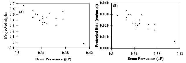
Figure 2. (A) Shows the baseline  $\alpha$  and (B) the baseline  $\beta$  parameters projected to the 50-keV triode extractor installed on the prototype injector. Calculations based on these measurements are used in the 1.25 MeV cw RFQ calculations.
