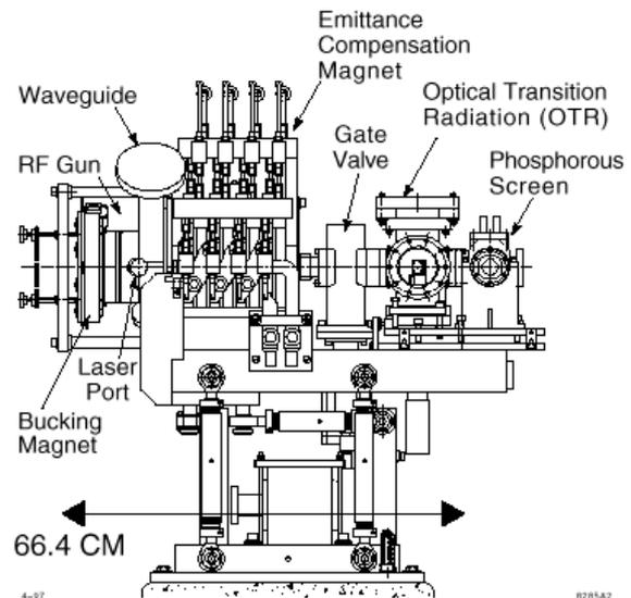
Figure 1: Layout of the ATF photoinjector.
