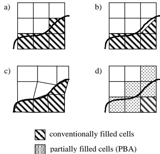
Figure 1: Grid approximations of rounded boundaries: Standard (a), triangular (b), non-orthogonal (c), PBA (d)
