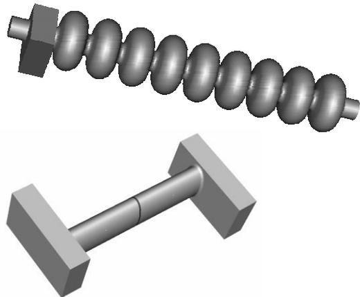
Fig. 4: TESLA 9-cell cavity with planned input coupler structure.
