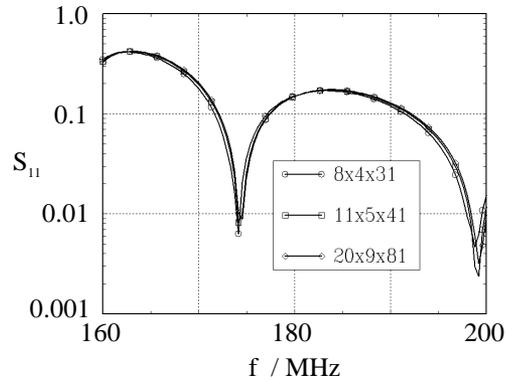
Fig. 3: Twisted Waveguide: reflection coefficient  $S_{11}$  for different grid resolutions
