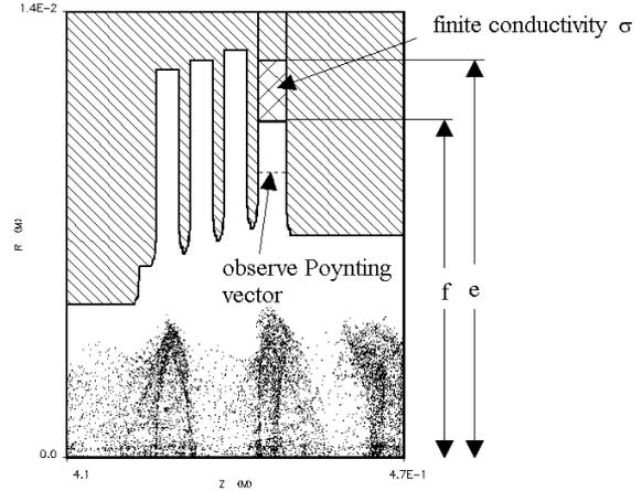
Figure 4: An example of MAGIC2D simulation. A finite conducting material is set in the coupler region to match  $S_{11}$ . Output power is calculated by time average of the area integral of Poynting vector. This structure is KEK XB72K#9 output cavity.
