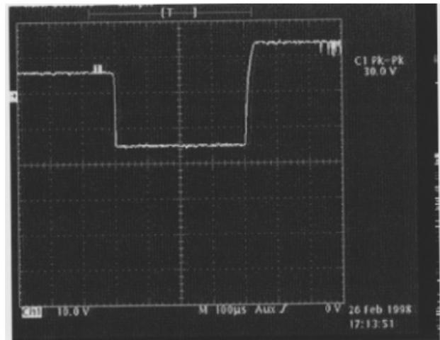
Figure 1: Stable oscillation in the wavelength of around 24  $\mu\text{m}$ . The pulse duration is continued over 0.4ms, the beam current ranging from 2 to 4mA, and the maximum laser power about a hundred watts in average.
