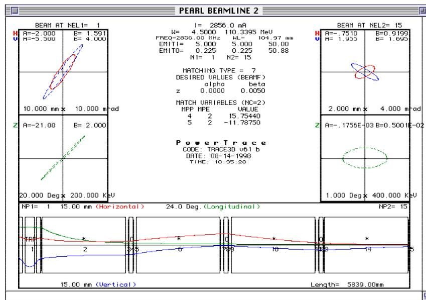
Figure 2: Pulse Compression with Four Accelerator Sections
