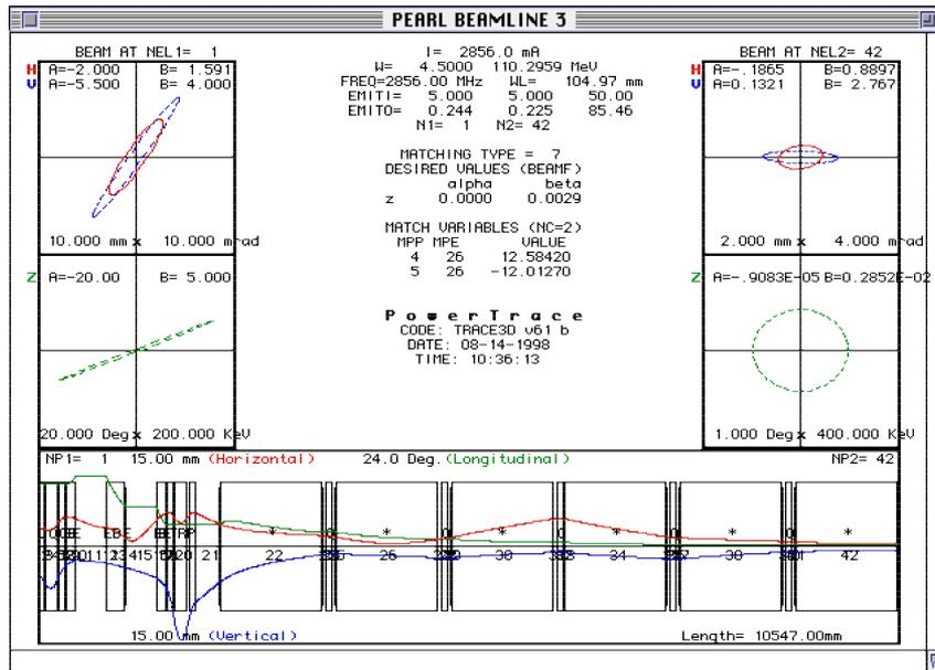
Figure 3: Pulse Compression with Magnetic Chicane Buncher and Six Accelerator Sections
