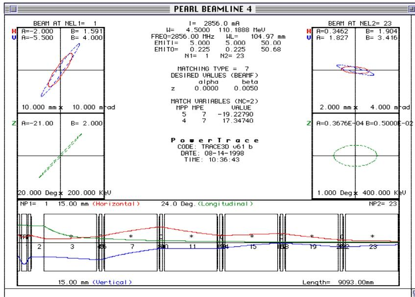
Figure 4: Pulse Compression with Six Accelerator Sections
