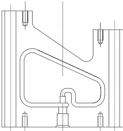
Figure 7: One way cooling channel of the endstems.
