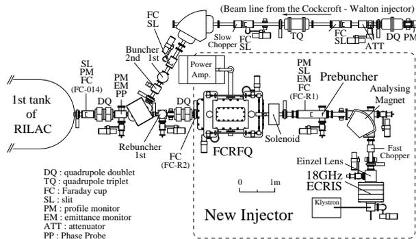
Figure 2: Schematic drawing of the new injector.
