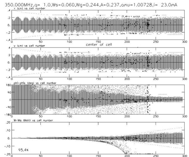
Figure 3. PARMTEQM simulation of the RFQ using 5000 particles. From top to bottom are: x, y, phase, and energy coordinates versus cell number. Bold black points indicate lost particles in the RFQ.
