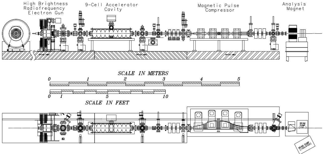
Figure 1: Layout of photoinjector components
