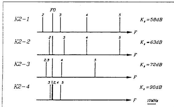
Figure 5: Diagram of cavity detunings for all versions of the klystron.
