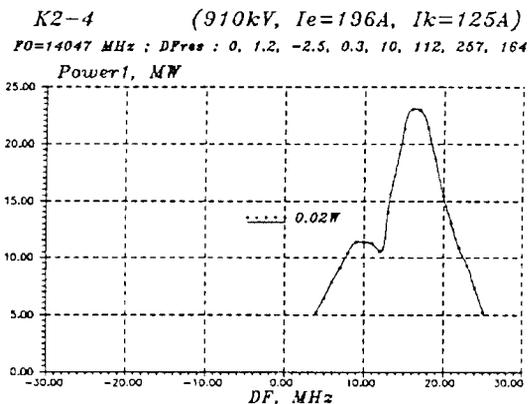
Figure 8: Amplitude-frequency characteristic of the klystron.
