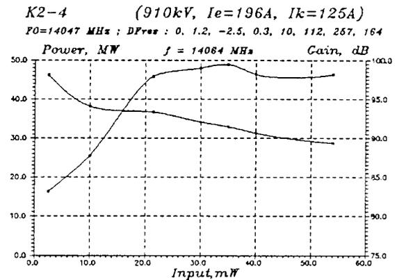
Figure 7: Amplitude characteristic of the klystron.
