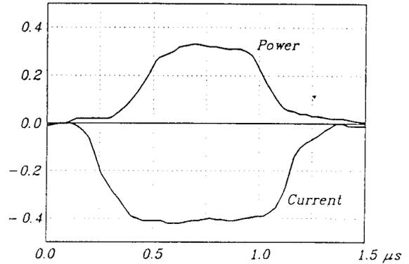
Figure 6: RF pulse envelopes for output power and collector current of the klystron.
