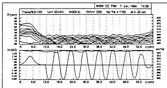
Figure 3: Transverse dynamics of the beam.
