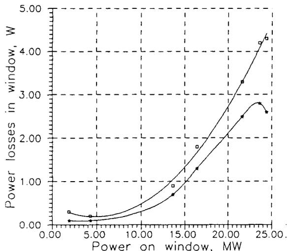
Figure 9: Power losses in the output window.
