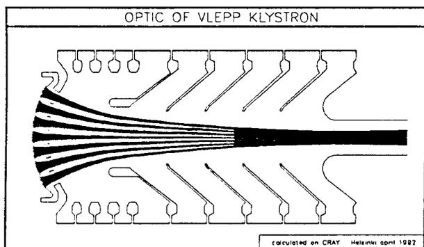
Figure 2: Optics of electron gun.
