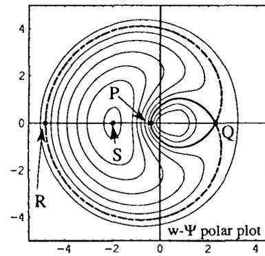
Figure 5: Polar plot of  $w$  vs.  $\Psi$  for the trajectories corresponding to the parametric resonance with  $\Delta = 0.35$ ,  $L = 0$ ,  $\epsilon = 0.3$ .
