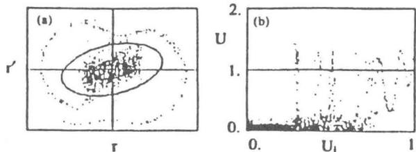
Figure 2: Results at 20 plasma periods from multiparticle simulation of an initial Gaussian-density laminar beam in a uniform linear focusing channel. The initial rms size in  $x$  is larger than the matched value by a factor  $M = 1.5$ . We show a)  $r - r'$  phase space, b) particle energy  $U$  versus the initial particle energy  $U_i$ .
