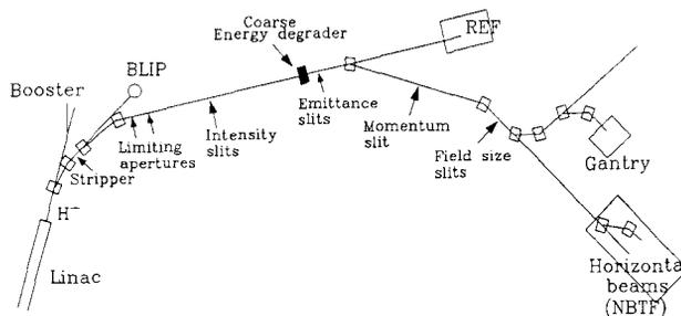
Fig. 1. Schematic of transport lines to therapy facility.
