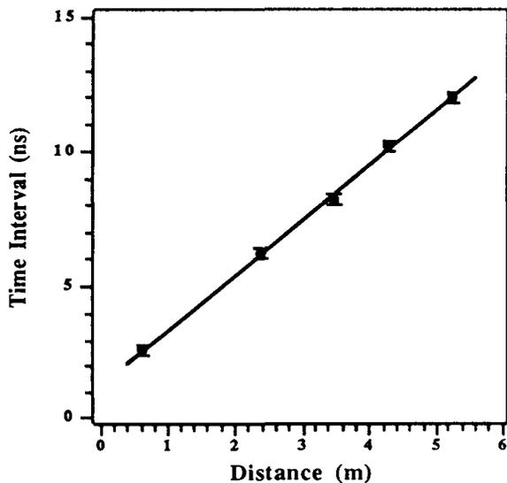
Fig. 3. Time interval between two space-charge waves vs. drifting distance, as measured by the five current monitors. The solid line is a least-square fitting of the experimental data.
