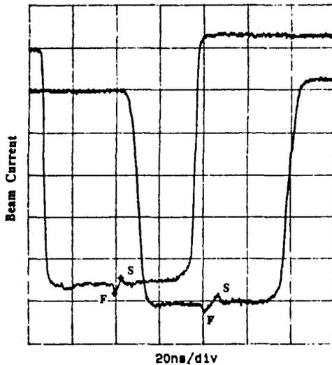
Fig. 1. Beam current signals modulated with localized perturbations showing the amplitude, polarity, and separation time of two space-charge waves.
