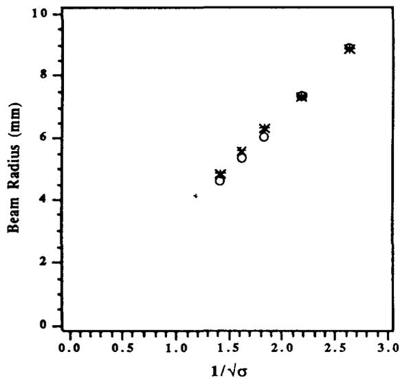
Fig. 4. Comparison of the measured beam radii from two different approaches: the stars are from the space-charge wave method, while the circles are from the beam image identifier, where  $\sigma$  is the phase advance of betatron oscillation with space charge.
