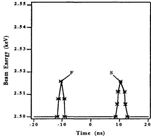
Fig. 2. Energy spectrum of a beam with localized space-charge waves.
