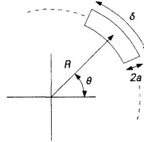
Fig. 1 Bunch of length  $\delta$  and radius  $a$  in bend of radius  $R$ .
