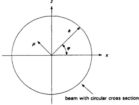
Fig. 2. Geometry used for the beam's local coordinate system. The beam is moving out of the plane of the page.
